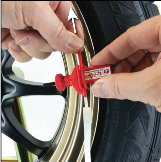
Feed it through the guide channel (the slot between the control ring spool and the bridge).
