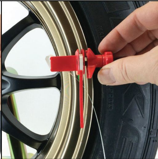
Feed it up and over the spool so it hangs down just past the spool. NOTE: The tool has been turned over in this picture to illustrate.
