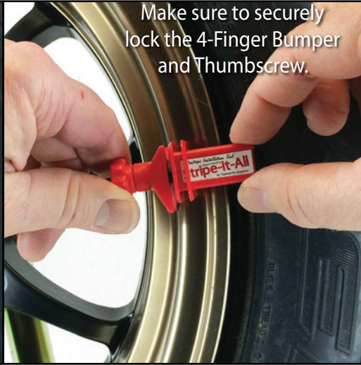
Determine where you want the rimstripe to be installed. Then adjust and lock the 4-Finger Bumper.
