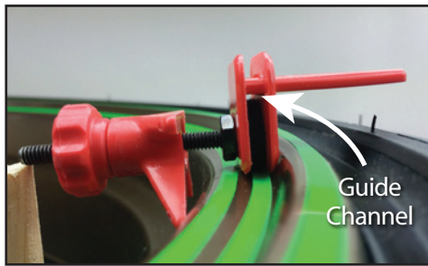
Middle Rimstripe Installation
