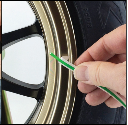
Take one of the rimstripes and separate it from the backing paper to expose approximately 1/2 inch of adhesive.
