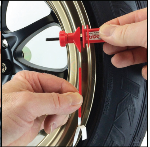
Make sure the Easy Feeder is turned so the adhesive side of the tape is facing outward.
