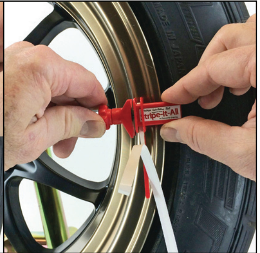
Initial Contact: Carefully make edge contact with the bumper and then press the tool and exposed tape to the wheel.
